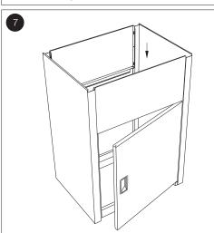
Align the second Front/Rear Head Panel (2) with the Side Panels (1) and slide over the Door Hinge Rod (6). Snap the remaining two Panel Fixing Clips (3) into position.
