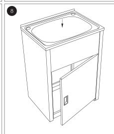
Install Waste and Bypass fittings supplied with Tub. Position Tub (8) on top of the Cabinet. Assembly.
