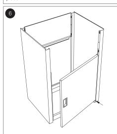
Align and insert the Door Assembly (7) with the corresponding holes in the Hinge Base (5).
