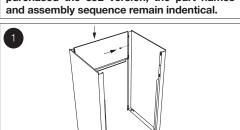
Slide one Front/Rear Head Panel (2) onto Side Panels (1) and snap Panel Fixing Clips (3) into place.
